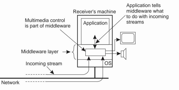
The principle of synchronization as supported by high-level interfaces.
