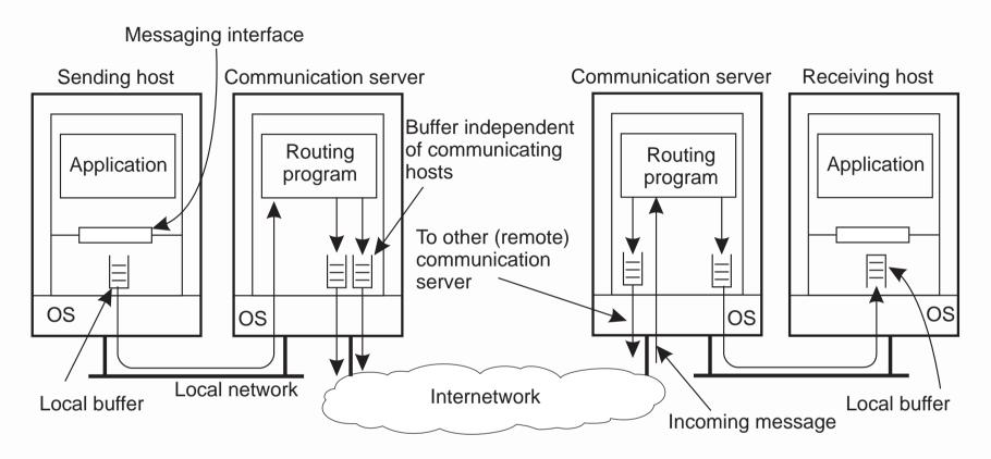
Organization of a communication system, hosts connected through a network
