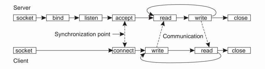
The general pattern followed by a client and server for connection-oriented communication using sockets.
