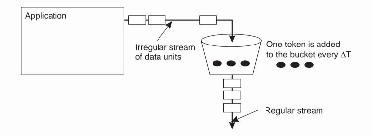
The principle of a token bucket algorithm
