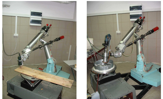
(a) RNT robot milling in wood (b) RNT robot polishing metal
