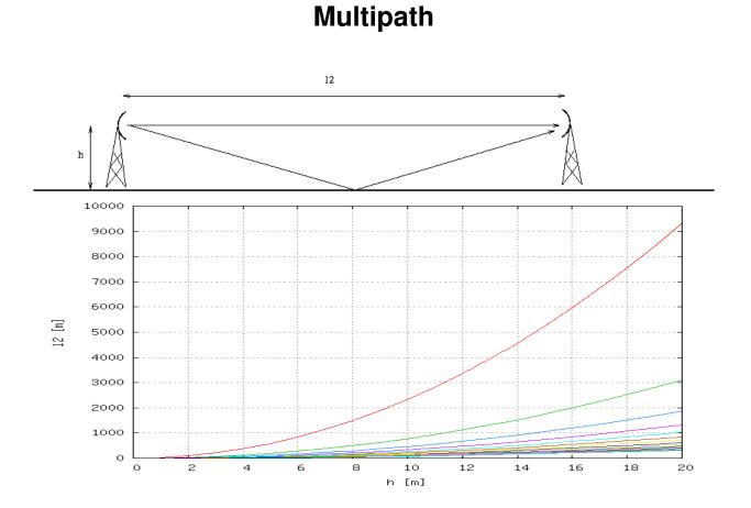
(I2=distance vs. h=tower height), 7GHz, curves for [1 3 5 .. 15]\*lambda/2, flat earth geometry
