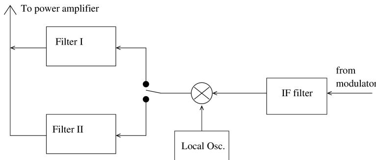
1. A dualband transmitter (sketched above) is to work in UMTS-FDD standard in two USA uplink channels with frequencies 1850-1910 MHz (band II) and 1710-1755 MHz (band IV).
