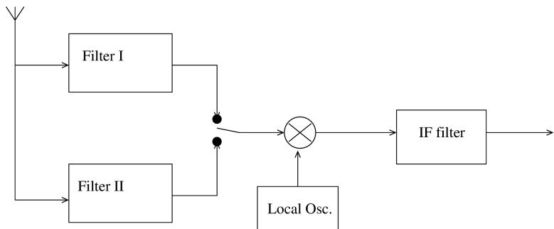
1. A dualband receiver (sketched above) is to work in UMTS-FDD standard in EU and USA downlink channels with frequencies 2110-2170 MHz (EU) 1930-1990 MHz (US).
