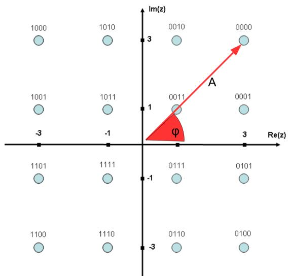
Constellation diagram: each 4 bits are mapped to one I/Q (or A/phi) pair
