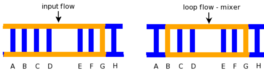
Figure 3. Typical operations of lab-on-a-chip: on the left the input solution flow, on the right the cycle flow in the microfluidic processor
