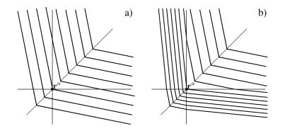
Fig. 1. Isoline contours for the analytic scalarizing achievement function (2): a) with partial achievements (5), (b) with partial achievements (4)
