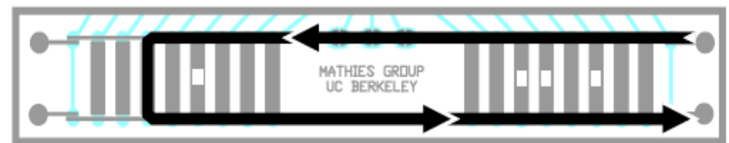
(B) Load input DNA into fluidic loop and chamber
