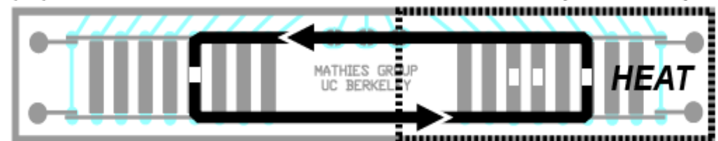
(D) Release and transfer DNA to next capture step
