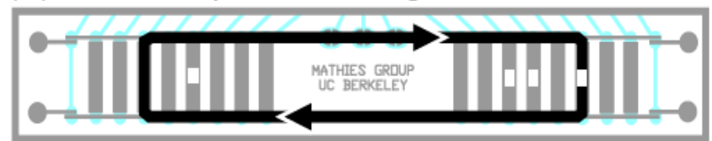
(C) Circulate input DNA through selected beads
